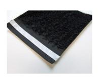
Structural underlays are designed to provide micro ventilation to the underside of the zinc, drain away any moisture, and offer acoustic absorption properties. They are specifically designed for use under fully supported traditional metal roofing and cladding. The extreme elasticity of the monofilaments that make up the spacer mat allows excellent sound absorption, significantly decreasing rain drumming noise.
